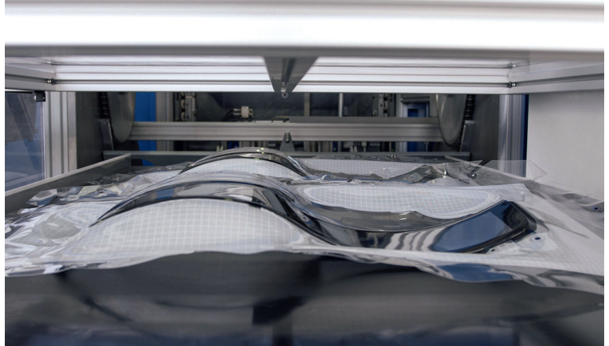
Fig. 2. The FIM machine for 3D heat forming of large-size polycarbonate arcs operates at 60 bar
