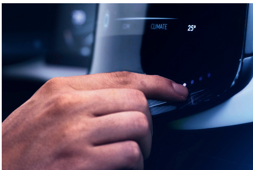
Fig. 4. Surface topographies on the panel make blind operation of functions in the display easier (© Continental)
